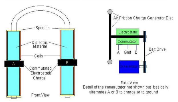
Static Electricity that is generated on a properly treated insulated wire will produce more than a kilowatt in a light wind, according to Paul Clint. This becomes possible because of a phenomenon in physics known as the electret effect.
