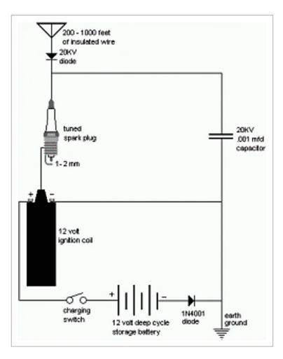
batteries. An efficient voltage controller must be used to keep your battery from overcharging. The least expensive design used a spark plug, an old automotive coil, a 0.001 uF, 3 to 20 kV capacitor and a ground rod.
