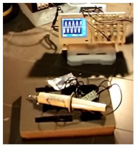
The name of the HV probe at the bottom is Tektronix P6015A, so we know there is high voltage involved. Tastkopf 1000:1, 3 pF,100 MOhm
