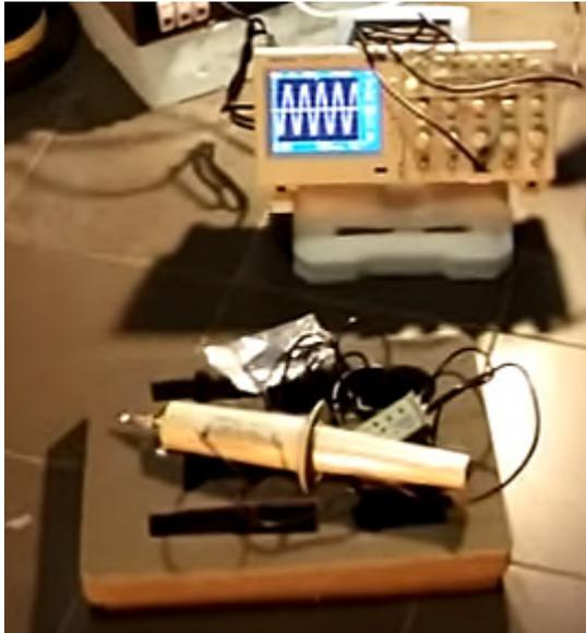
The name of the HV probe at the bottom is **Tektronix P6015A**, so we know there is high voltage involved. Tastkopf 1000:1, 3 pF, 100 MOhm
